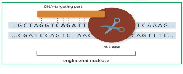
**Figure 1.** Each Zinc Finger Nuclease (ZFN) consists of two active domains: a.) A DNAbinding domain composed of a series of two finger modules, each recognizing a unique hexamer sequence (6 bp) of DNA. Two finger modules are put together to form Zinc Fingerprint Protein, each with  $\geq 24$  bp special properties. b.) The DNA-cleaving domain formed by the nuclease domain of Fok I. When DNA-binding domains and DNA-cleaving are combined, a highly speculative pair of 'genomic scales' is created.
