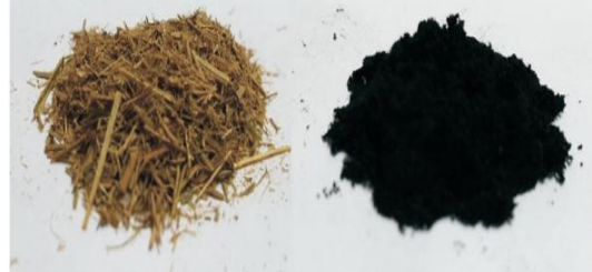
Fig. 7: Biochar production using rice stubble
