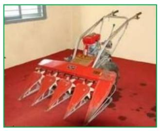
• These types of reapers are suitable for crops like wheat and rice. In this reaper there is no shattering of the crop.
