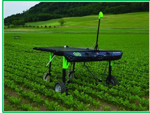
Fig. 2. Mechanical weeding through Agri-robots in vegetable crops
