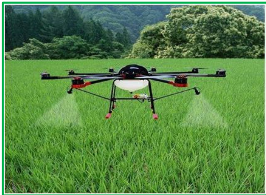
Fig.3. spraying of insecticides through drones in paddy field
