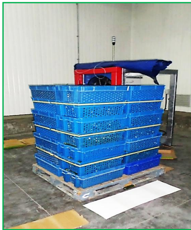
Fig.03. Heat removal from cucumbers using Forced-Air Cooling
