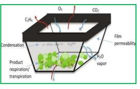
carbon dioxide. Therefore, whenever required, the balance of modified atmosphere is created with nitrogen.
