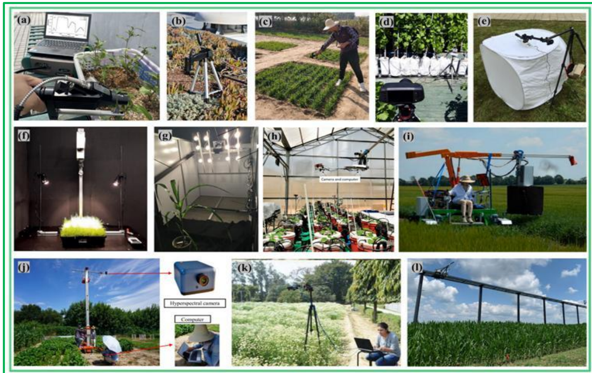
Figure 2: Proximal hyperspectral sensor setups for abiotic stress monitoring in plants under laboratory and field conditions
