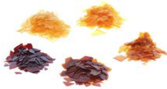
Resin secreted by the female lac bug on trees is processed and sold as dry flakes
