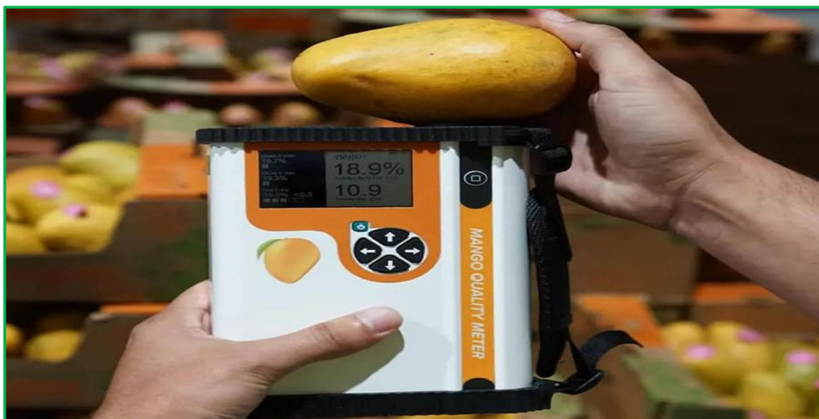
Image 1. A mango being measured for quality parameters using a mango quality meter device during post-harvest assessment
