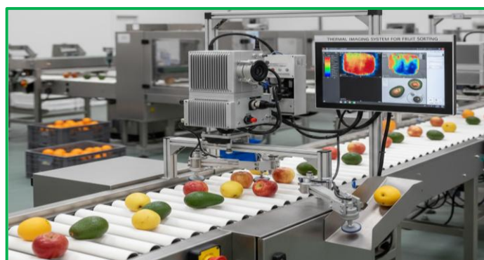
Figure 3. Thermal imaging system integrated into a postharvest sorting line.
