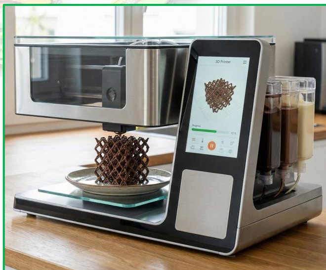
Figure 1. A modern 3D food printer is constructing a customised food item layer by layer.
