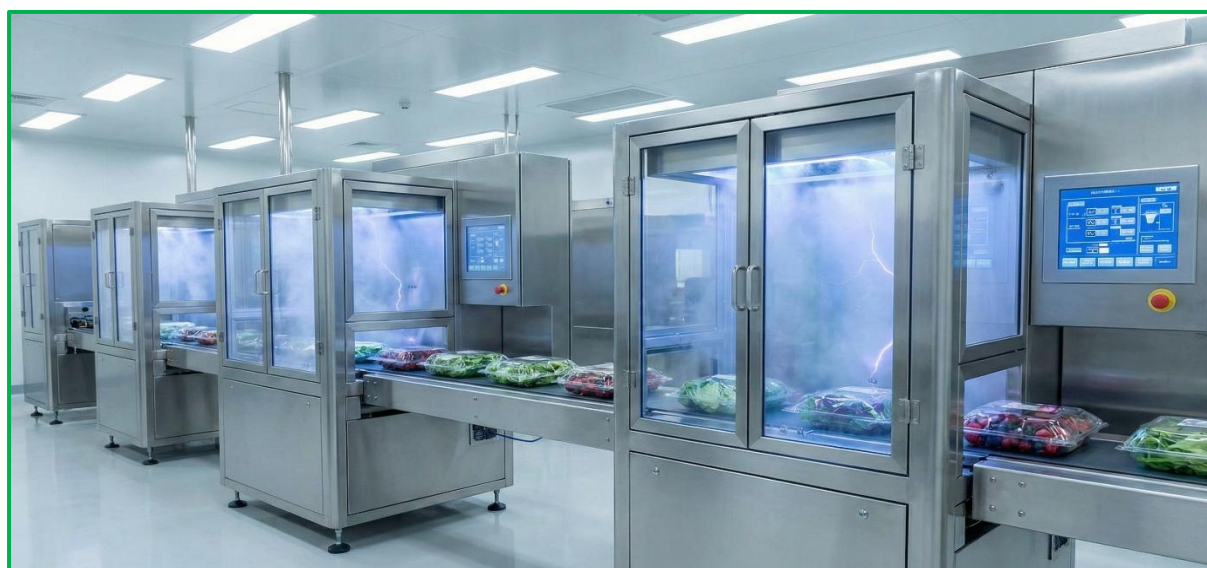
Figure 3. Cold Plasma System Integrated in Processing Line
