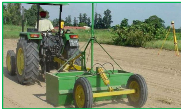
Fig.1: Tractor-operated laser land levelling.
