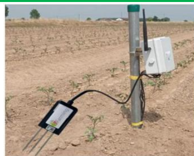
2. Soil nutrient/NPK sensor; Use as: Figure: Soil nutrient sensor for site-specific nutrient management.
