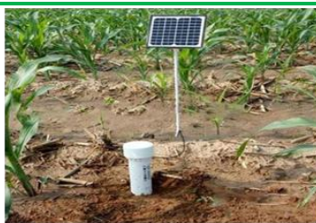
1. Soil moisture sensor in a crop field; Use as: Figure: Soil moisture sensor for real-time monitoring of soil water status in precision agriculture
