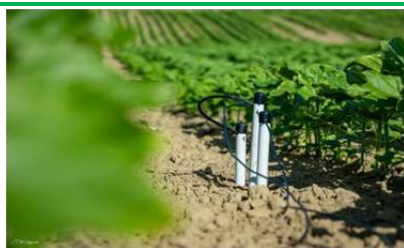
1. Soil moisture sensor in a crop field; Use as: Figure: Soil moisture sensor for real-time monitoring of soil water status in precision agriculture
