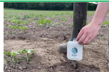
1. Soil moisture sensor in a crop field; Use as: Figure: Soil moisture sensor for real-time monitoring of soil water status in precision agriculture
