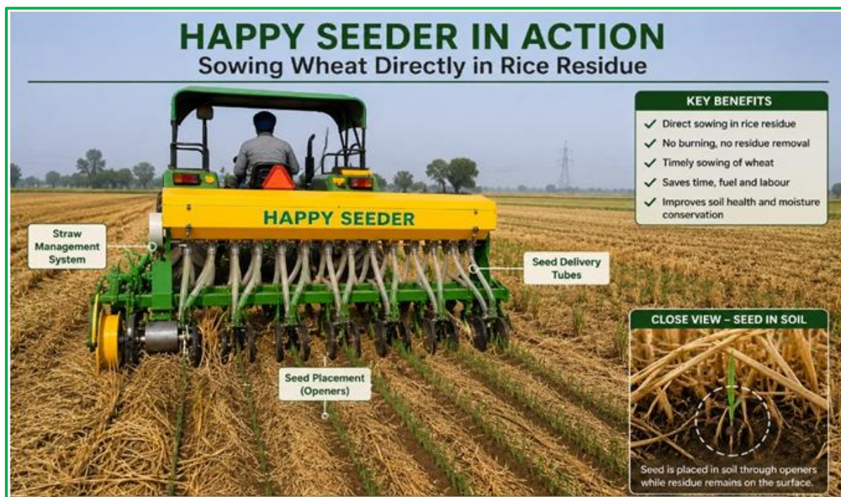
Fig. 2: Use of Happy Seeder for sowing wheat directly into rice residues
