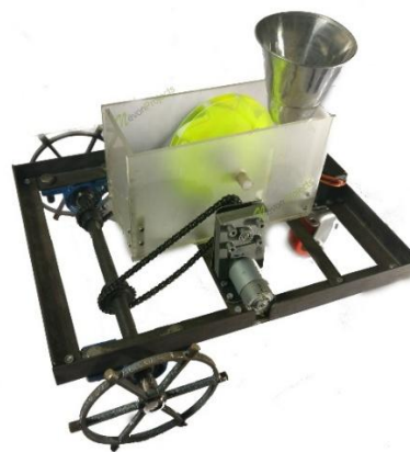
Fig 2: Smart Seed sower rover https://nevonprojects.com
